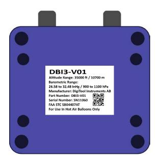
Attach bracket e.g. belt-loop part to instrument using the four mounted pan-head M4 screws, 1 thru 4. Screw head is TORX T8.
